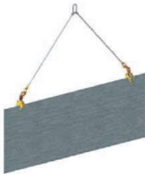
LIFTING LONG PLATE WITH A 2 LEGGED CHAIN SLING
